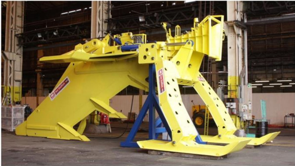
Plate 3-2: Sea Stallion Cable Plough (Photo Credit: Boskalis)
