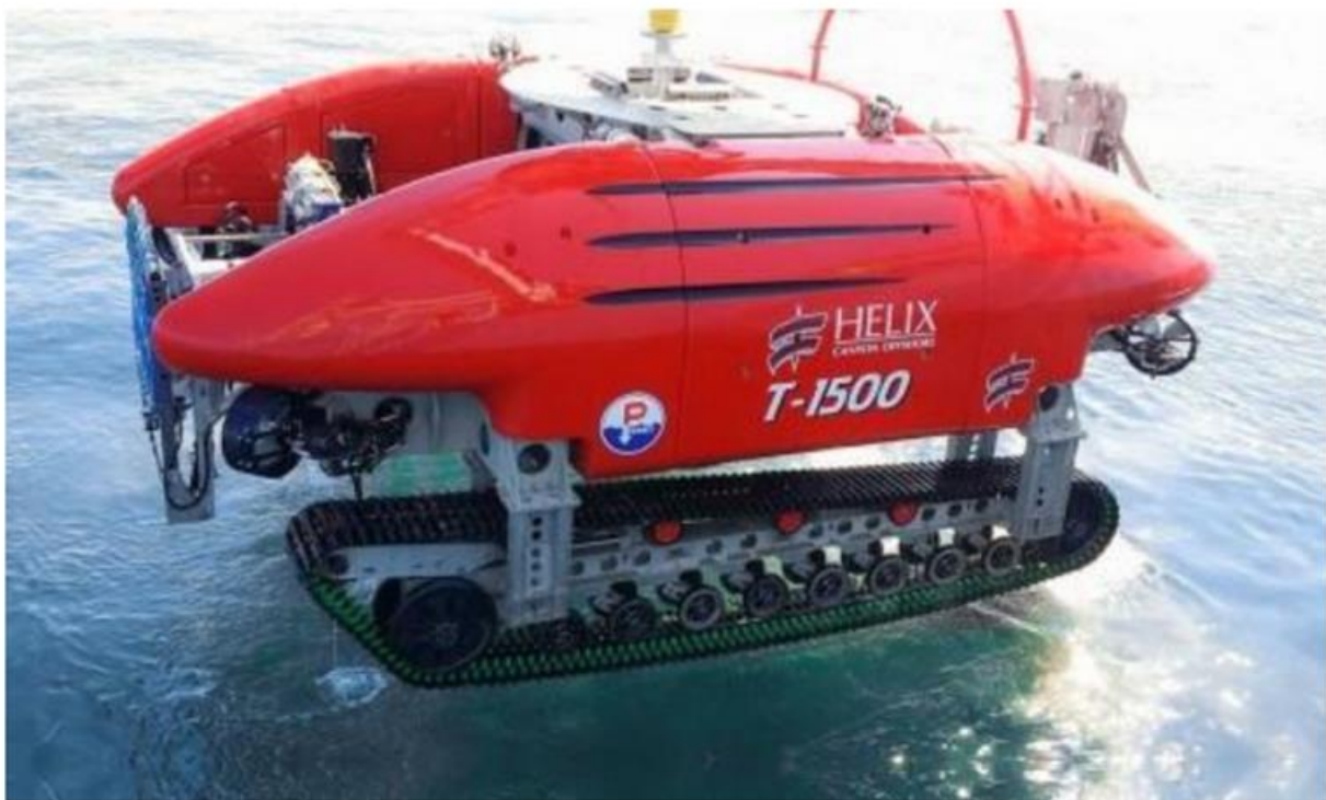
Plate 3-4: Example of a Water Jet Trenching Tool (Photo Credit: Helix Energy Systems)
