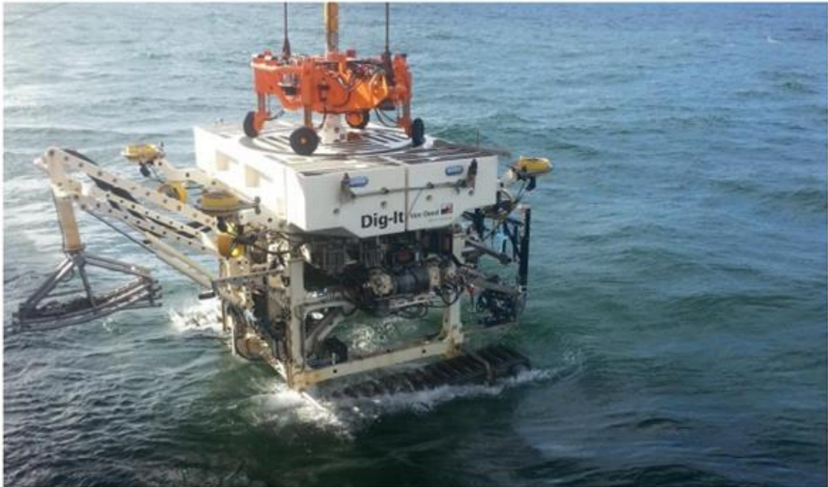
Plate 3-7: Q Series Trencher (Photo Credit: Van Oord)
