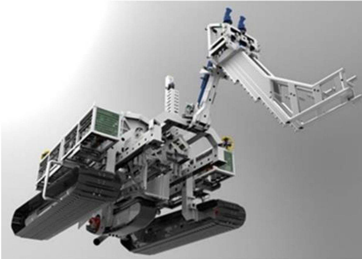
Plate 3-8: Cable Burial Tractor/Hybrid Trencher (Photo Credit: Prysmian Group)
