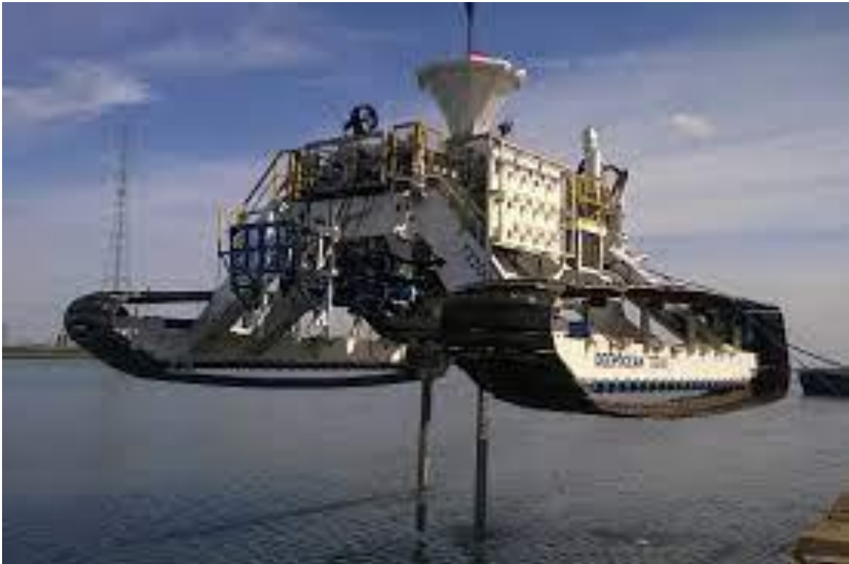
Plate 3-5: Example of a Mechanical Trencher (Photo Credit: DeepOcean)
