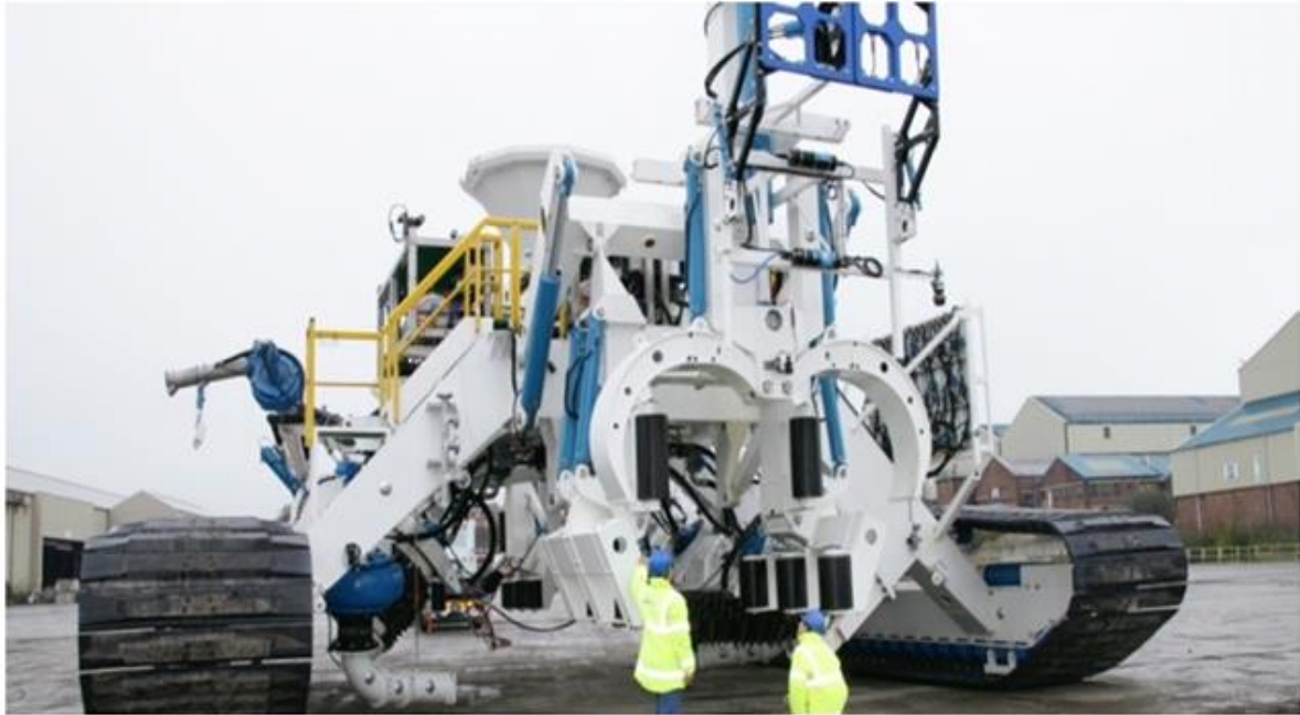
Plate 3-9: Helix Robotics Solutions i-Trencher (Photo Credit: Helix Energy Systems)
